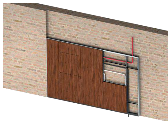
Perimeter / False Wall
